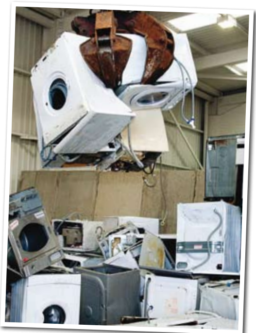
Above: Washing machines being baled and crushed at the new WEEE facility in Ballymount, South County Dublin.
